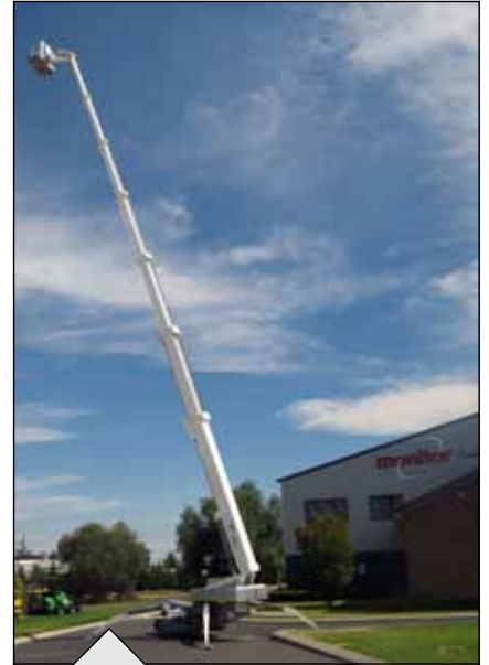
Horizontal outreach is now up to a huge 14 metres. (or 12.3m with 250kg).
