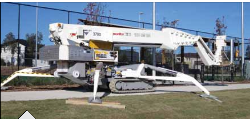
Like most of the Ommes in Australia, the 3700RBDJ is a dual power machine, combining a powerful 3 cylinder water cooled Kubota diesel engine with a double-sized battery system.
