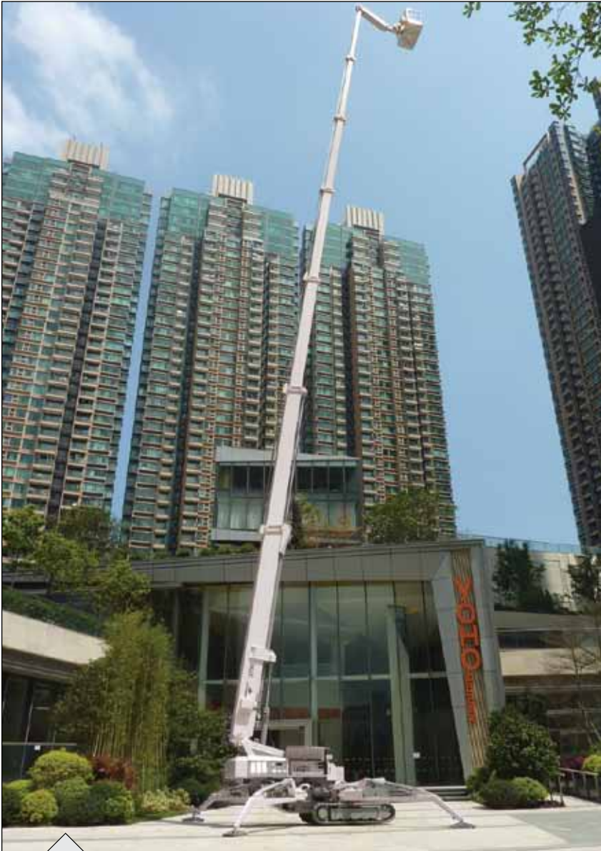
Weighing only 5.3 tonnes, this Omme is incredibly light for a machine that provides a 37m working height and an increased S.W.L. of 250kg.
