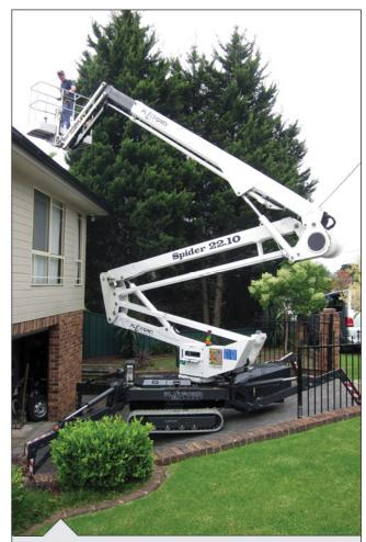
Excellent up-and-over reach with modern double knuckle technology, and adjustable fly-jib for extra manoevrability. The 2210 also has the most unique ability to rotate a complete 360° even when the stabilizer legs are set in their narrow position.
