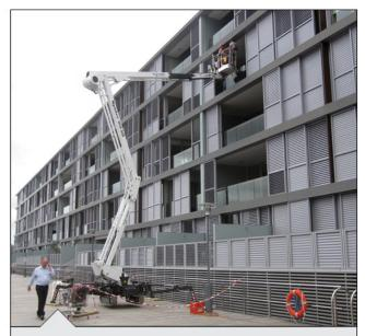
Weighing only just over 3 tonne, this 22m spider is ideally suited for use on load-sensitive surfaces, such as the boardwalk pictured above.
