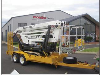
Compact dimensions + light weight = transportability! The 2210 is available on a very strong tilt-bed trailer weighing in at under 4.5 tonnes.
