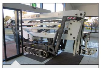
With the basket removed and tracks in narrow position, the 2210 allows for doorway access.
