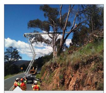
The radio control feature allows all functions to be controlled from the basket (or any other position). This includes driving, setting the stabilizer legs and operating the booms, making the 2210 exceptionally operator-friendly.
